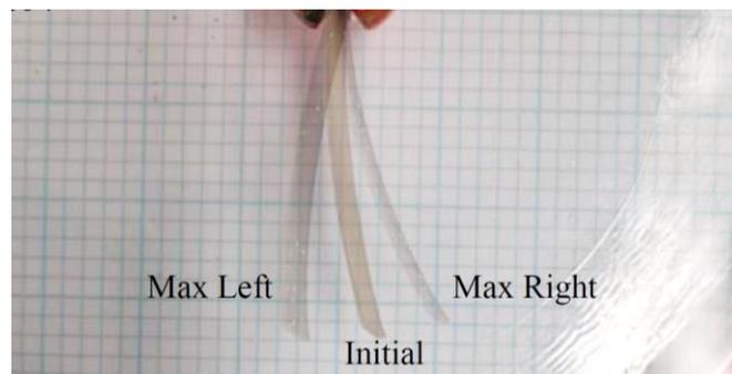
Figure 2. Reversible actuation of a DLP fabricated cation conductor polymer membrane
