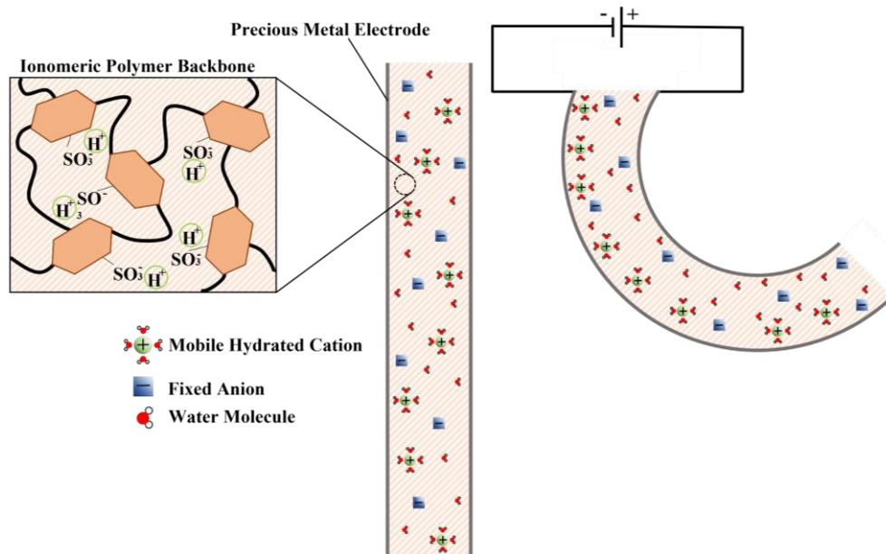
Figure 1: Schematic of the actuation mechanism of the IPMC membrane materials. Reproduced from K. E. Engel, P. A. Kilmartin, O. Diegel, *Polymer Chemistry* **2022**.
